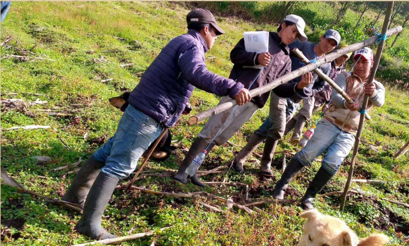
Farmers from the Manzano Guaranguí community of the Ibarra district using Level A to draw contour lines in a workshop on soil conservation practices.
